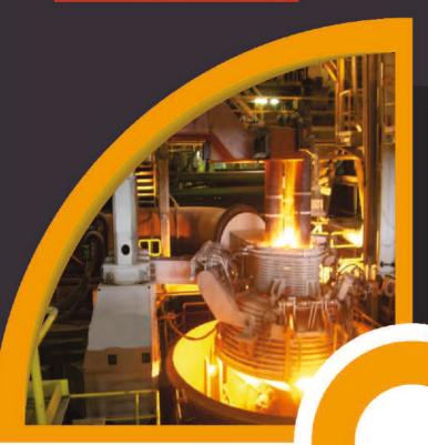
Ladle Refining Furnace and Ethern Mr. Furnace
